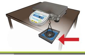
Then, with Nimbus placed on a tabletop with a cutout, the sample is **placed in a basket** attached to the balance's weigh-below hook and **lowered into a container of water** below.
