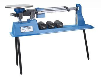
Created to withstand daily student use, Adam Equipment's patented TBB triple beam balance offers the best value for teaching mass measurement concepts. With rugged construction and security slot to prevent theft, the durable TBB is ideal for classroom environments. Other features include sturdy tripod legs for density measurement, weigh-below hook, magnetic damping for faster stability, notched and tiered graduated beams with center reading, and holders for storing extra weights.
